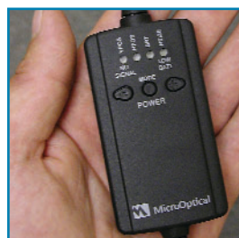
Belt-Worn Battery Dimensions: 3" x 2" x 0.5"
